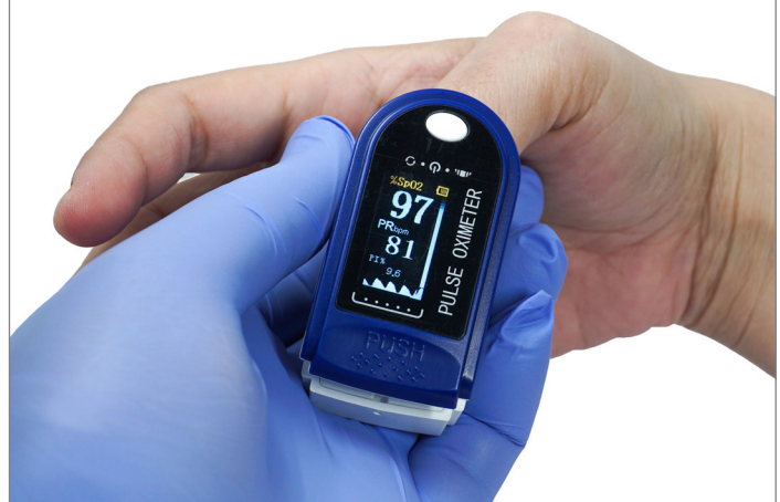
Figure 2: A portable oximeter is used to measure oxygen levels and pulse rate. Portable, low-cost life science devices particularly benefit from incorporating colour glass filters.
