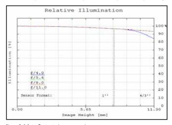
Figure 2: Relative illumination (center to corner)
