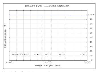
Figure 2: Relative illumination (center to corner)
