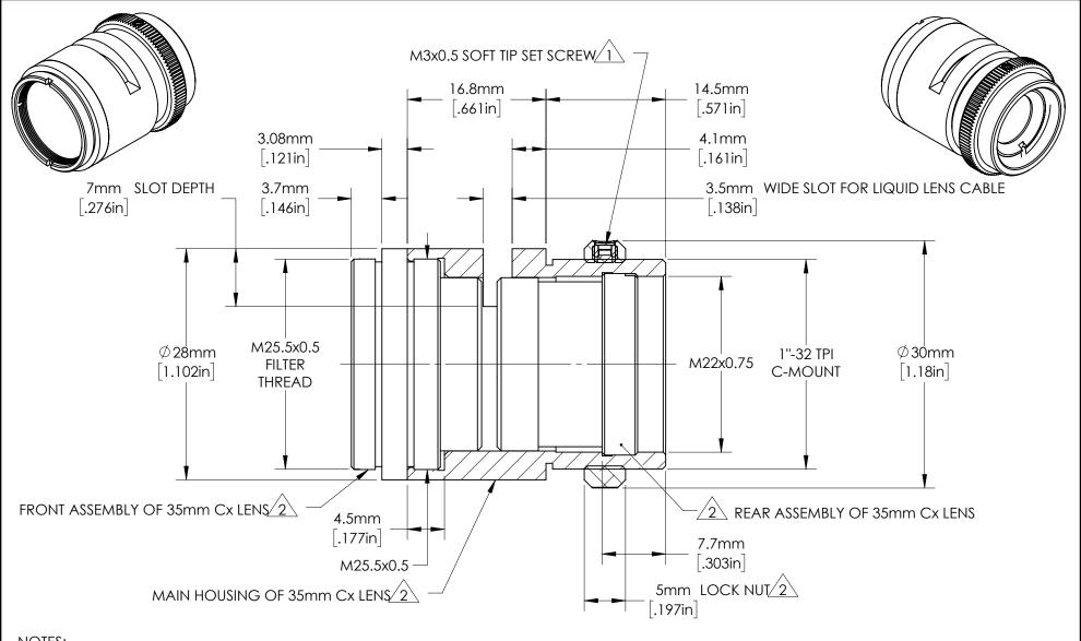
1.\ 3 m3x0.5 flat point stainless steel set screws included to optionally FIT 3 HOLES IN LOCK NUT, 120° APART.
