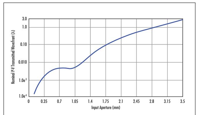
TECHSPEC® Scorpii™ Nd:YAG Beam Expanders are designed with diffraction-limited performance for a range of input beam diameters. These beam expanders are designed to increase the input beam diameter to a larger collimated beam. For custom wavelength and magnification combinations, please contact us.
