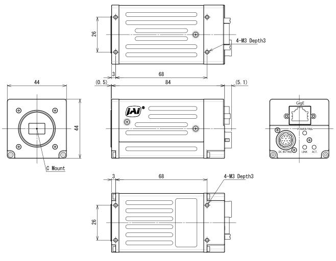
Dimensional tolerance:  $\pm 0.3$  mm Unit: mm
