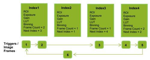
**1** Specify "1" in [SequencerSetStart], and start TriggerSequencer mode with index 1.
