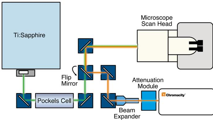
**Figure 2.** Laser and microscope optical setup. Beam path and intermediate optics for Ti:Sapphire and the Chromacity 1040 is shown above.
