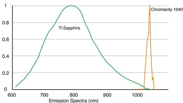
**Figure 1.** Emission Spectra of Ti:Sapphire and the Chromacity 1040.
