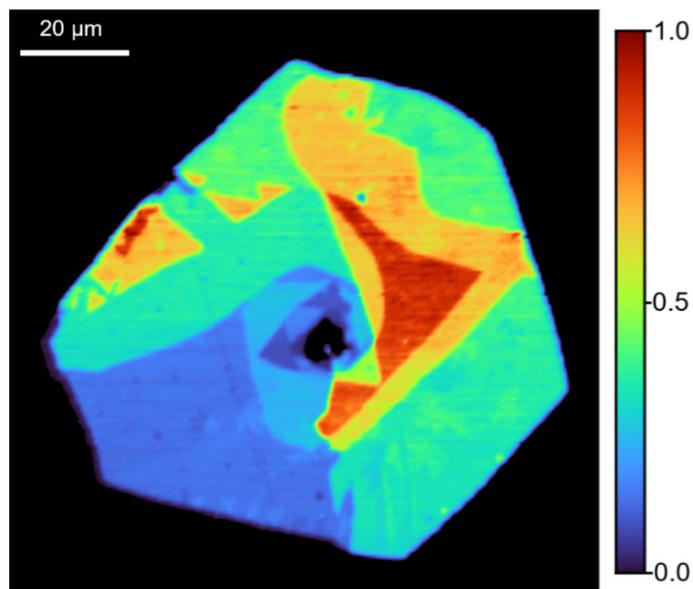
**FIGURE 4.** Second harmonic generation imaging of a WS<sub>2</sub> flake grown using CVD. The SHG imaging reveals that the flake is a polycrystal with each crystalline domain having a different SHG response due to differing number of layers, stacking symmetries and growth orientations.
