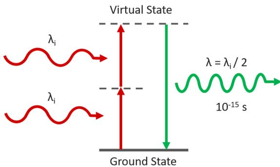
**FIGURE 1.** Schematic of the second harmonic process. This nonlinear optical process, causes two long wavelength photons to interact within a material to form new photons having twice the frequency of the input photons.
