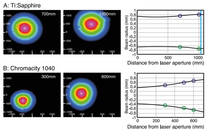
**Figure 3.** Laser beam profiles for Ti:Sapphire (A) and Chromacity 1040 (B). Blue lines on plots indicate relative position of focusing lenses for each laser beam path. Initial measurements showed the beam waist of the Chromacity 1040 to be narrower than the Ti:Sapphire but diverging much quicker. This divergence was compensated for in the final set up using a divergence adjustable beam expander.
