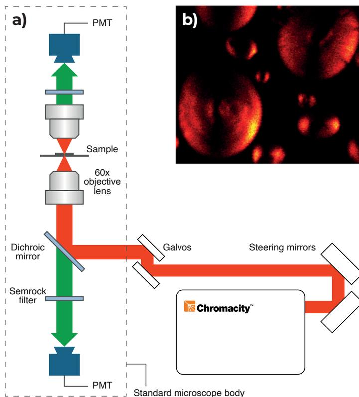
**Figure 3.** (a) Schematic representation of microscopy setup; (b) second harmonic generation observed in a sample of starch molecules. The field of view for this image is 100 x 100  $\mu\text{m}$ . Only 300 mW of laser light was necessary to acquire these images.
