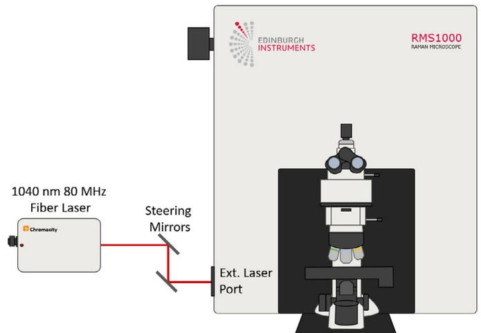
**FIGURE 2.** Example optical setup for SHG microscopy with the Edinburgh Instruments RMS1000. The laser excitation source is a Chromacity 1040 femtosecond fiber laser with an output wavelength of 1040 nm and a repetition rate of 80 MHz (Chromacity Ltd., UK).
