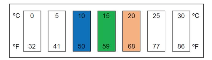
Liquid Crystal Thermometers are calibrated to turn green when the listed temperature is achieved. If green is not visible, the temperature will be midway between the elements that are blue and orange. Elements turn blue when they surpass their listed temperature and orange when they are just below their listed temperature.
