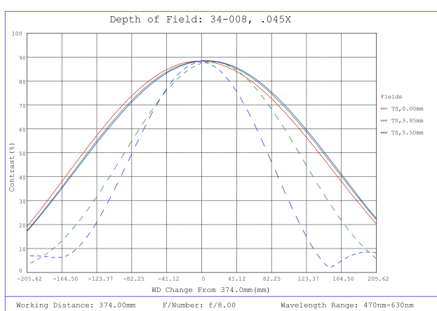
#34-008, 0.045X, 2/3" C-Mount TitanTL® Telecentric Lens, Depth of Field Plot, 374mm Working Distance, f8
