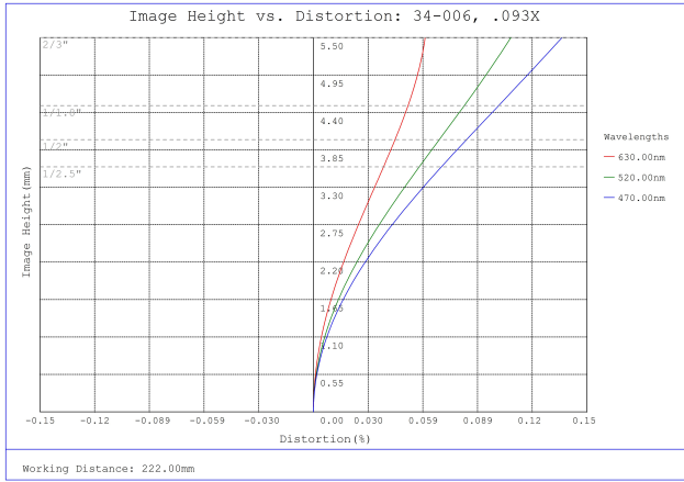
#34-006, 0.093X, 2/3" C-Mount TitanTL® Telecentric Lens, Distortion Plot
