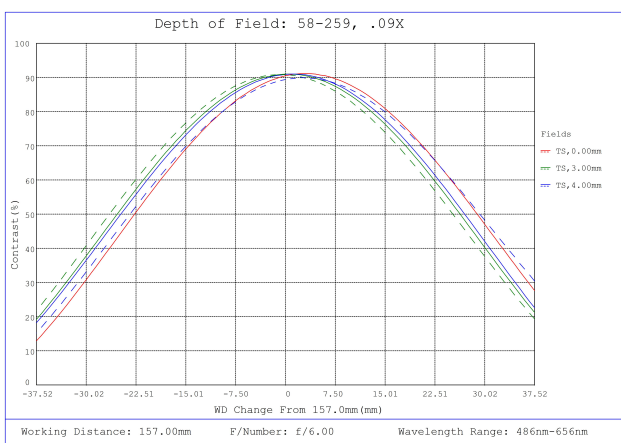
#58-259, 0.09X 1/2" GoldTL™ Telecentric Lens, Depth of Field Plot, 157mm Working Distance, f6
