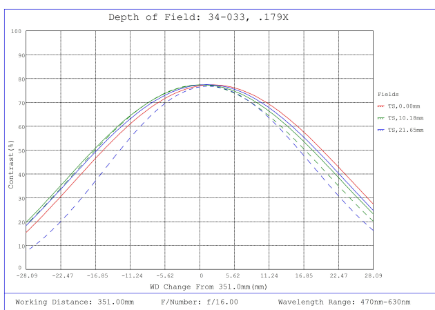
#34-033, 0.179X, 35mm F-Mount TitanTL® Telecentric Lens, Depth of Field Plot, 351mm Working Distance, f16
