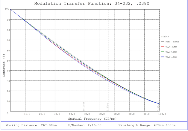
#34-032, 0.238X, 35mm F-Mount TitanTL® Telecentric Lens, Modulated Transfer Function (MTF) Plot, 267mm Working Distance, f16
