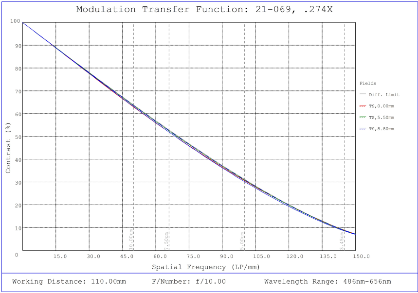
#21-069, 0.274X In-Line CobaltTL Telecentric Lens, Modulated Transfer Function (MTF) Plot, 110mm Working Distance, f10
