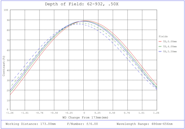
#62-932, 0.5X, 2/3" C-Mount PlatinumTL™ Telecentric Lens, Depth of Field Plot, 173mm Working Distance, f6
