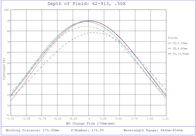
#62-913, 0.5X, 28.7mm M42 x 1.0 (6.56mm) PlatinumTL™ Telecentric Lens, Modulated Transfer Function (MTF) Plot, 175mm Working Distance, f6
