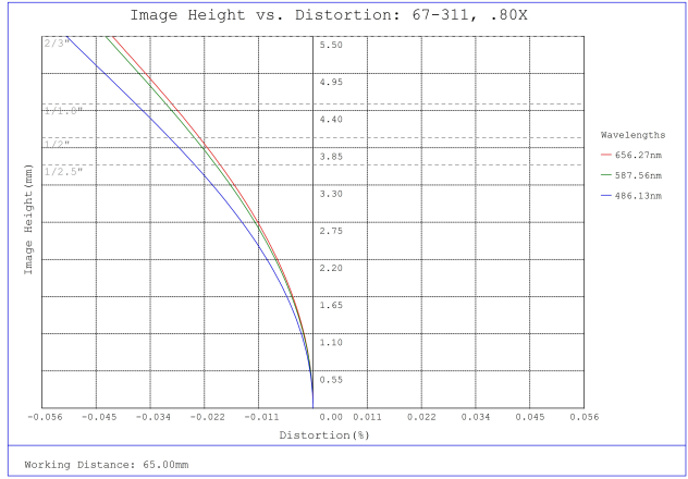
#67-311, 0.8X, 65mm WD, In-Line CompactTL™ Telecentric Lens, Distortion Plot
