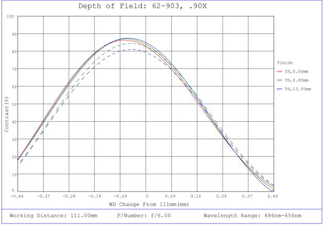
#62-903, 0.9X, 28.7mm M42 x 1.0 (6.56mm) PlatinumTL™ Telecentric Lens, Modulated Transfer Function (MTF) Plot, 111mm Working Distance, f6
