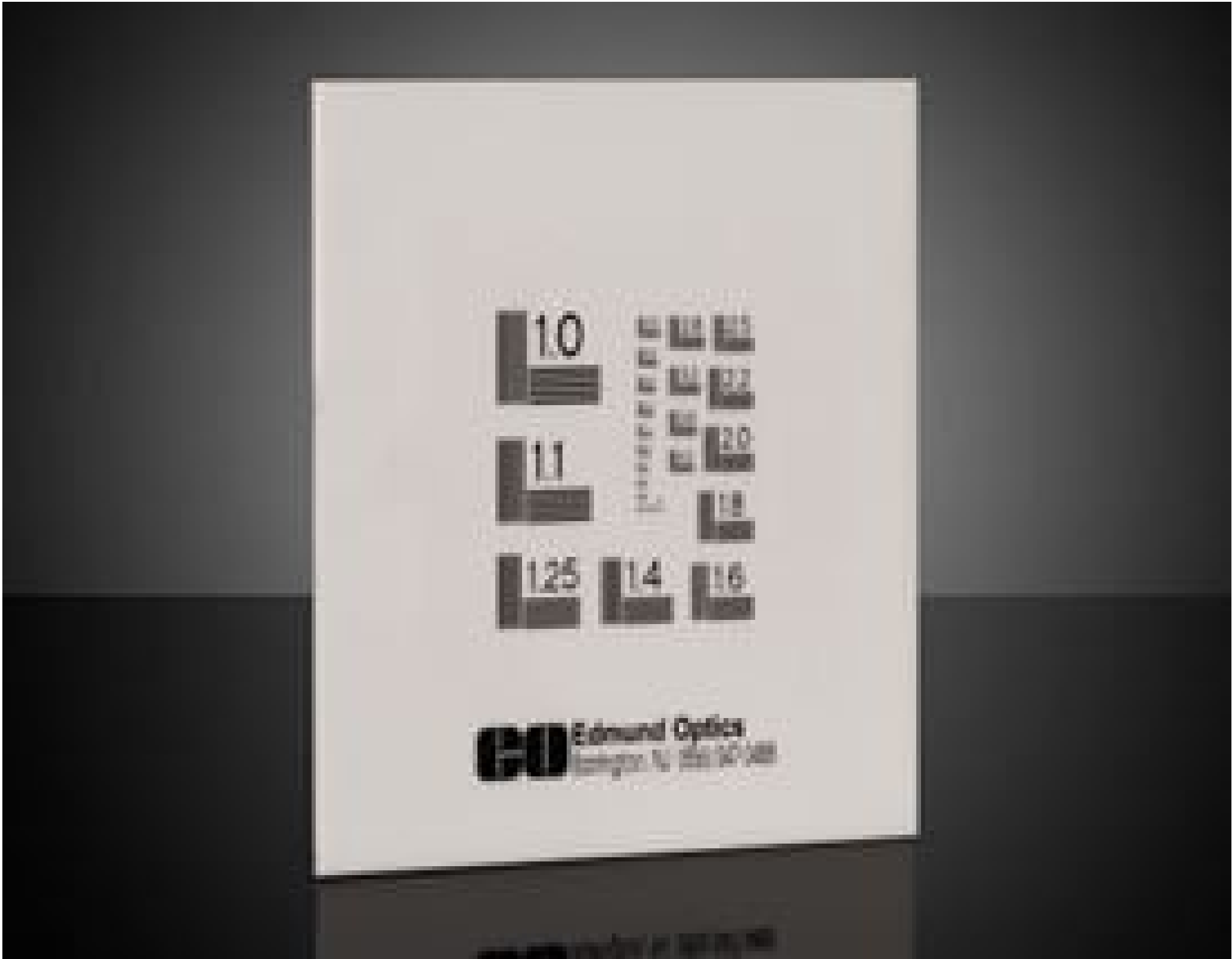
NBS 1963A Resolution Target
