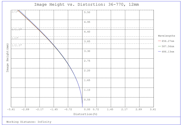
#36-770, 12mm f/11, 400-2000mm Primary WD, HRi Series Fixed Focal Length Lens, Distortion Plot
