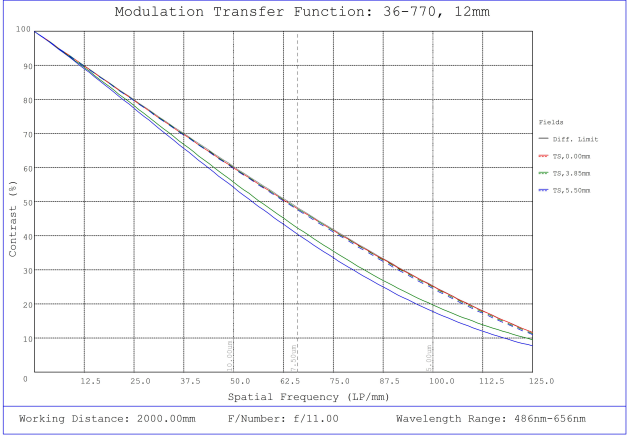
#36-770, 12mm f/11, 400-2000mm Primary WD, HRi Series Fixed Focal Length Lens, Modulated Transfer Function (MTF) Plot, 2000mm Working Distance, f11
