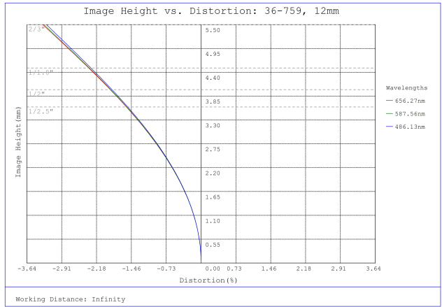
#36-759, 12mm f/2.8, 1000mm-∞ Primary WD, HRI Series Fixed Focal Length Lens, Distortion Plot
