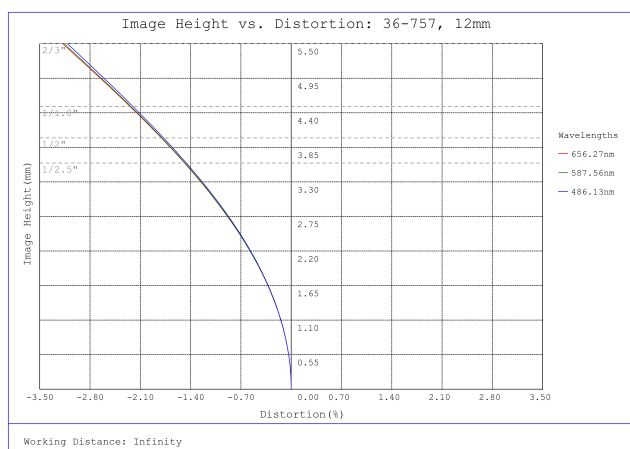
#36-757, 12mm f/2.8, 150-500mm Primary WD, HRi Series Fixed Focal Length Lens, Distortion Plot
