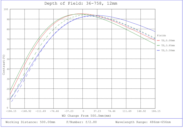
#36-758, 12mm f/2.8, 400-2000mm Primary WD, HRI Series Fixed Focal Length Lens, Depth of Field Plot, 500mm Working Distance, f2.8
