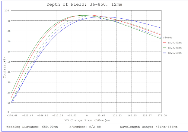
#36-850, 12mm f/2.8, 400-2000mm Primary WD, HRr Series Fixed Focal Length Lens, Depth of Field Plot, 650mm Working Distance, f2.8
