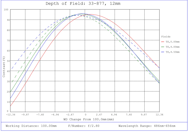
#33-877, 12mm, f/2.8 UCI Series Fixed Focal Length Lens, Depth of Field Plot, 100mm Working Distance, f2.8
