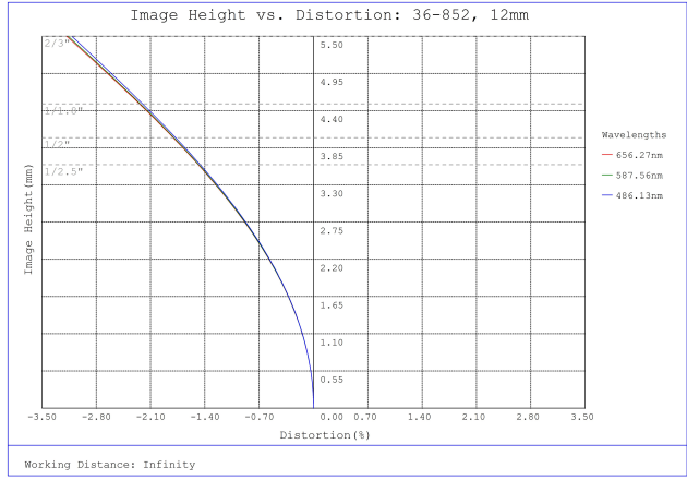
#36-852, 12mm f/4, 150-500mm Primary WD, HRr Series Fixed Focal Length Lens, Distortion Plot
