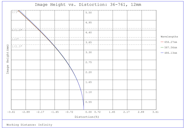
#36-761, 12mm f/4, 400-2000mm Primary WD, HRI Series Fixed Focal Length Lens, Distortion Plot
