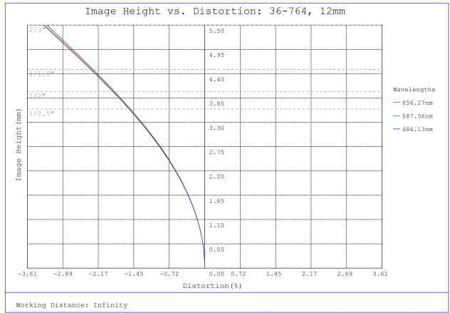
#36-764, 12mm f/5.6, 400-2000mm Primary WD, HRi Series Fixed Focal Length Lens, Distortion Plot
