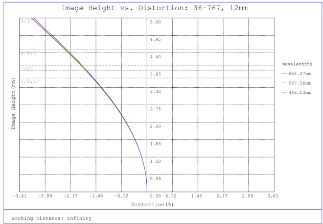
#36-767, 12mm f/8, 400-2000mm Primary WD, HRI Series Fixed Focal Length Lens, Distortion Plot
