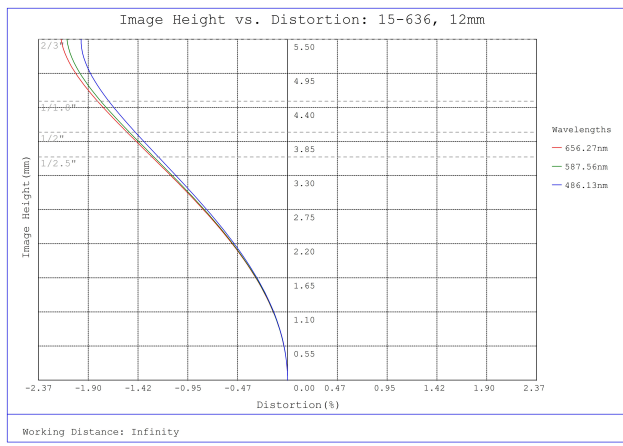
#15-636, 12mm, f/11 Cw Series Fixed Focal Length Lens, Distortion Plot
