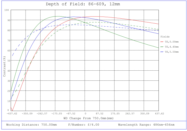
#86-609, 12mm, f/4 Ci Series Fixed Focal Length Lens, Depth of Field Plot, 750mm Working Distance, f4
