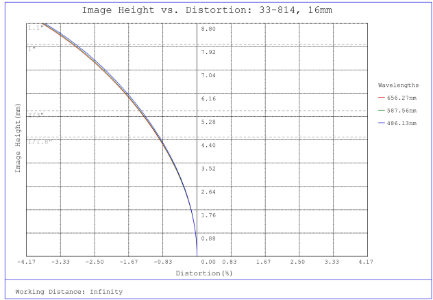
#33-814, 16mm f/1.8, HPI Series Fixed Focal Length Lens, Distortion Plot
