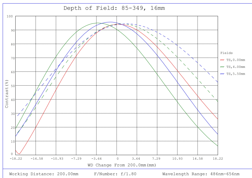
#85-349, 16mm, f/1.8 Ci Series Fixed Focal Length Lens, Depth of Field Plot, 200mm Working Distance, f1.8
