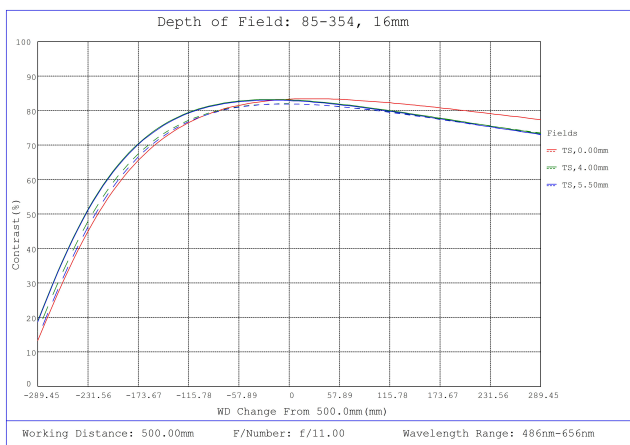
#85-354, 16mm, f/11 Ci Series Fixed Focal Length Lens, Depth of Field Plot, 500mm Working Distance, f11
