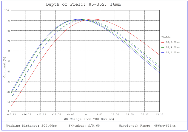
#85-352, 16mm, f/5.6 Ci Series Fixed Focal Length Lens, Depth of Field Plot, 200mm Working Distance, f5.6
