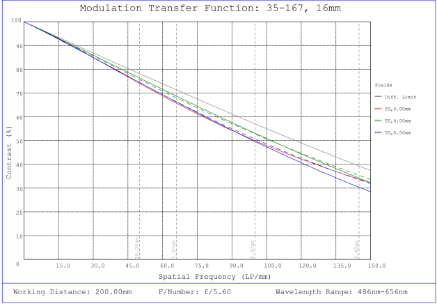
#35-167, 16mm, f/5.6 Cr Series Fixed Focal Length Lens, Modulated Transfer Function (MTF) Plot, 200mm Working Distance, f5.6
