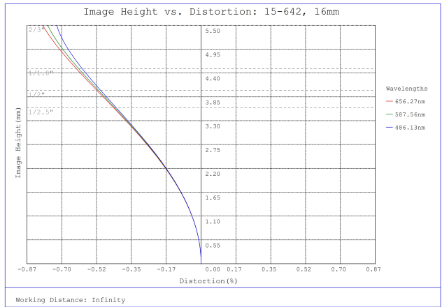
#15-642, 16mm, f/5.6 Cw Series Fixed Focal Length Lens, Distortion Plot
