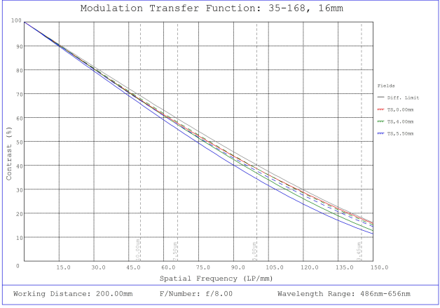
#35-168, 16mm, f/8 Cr Series Fixed Focal Length Lens, Modulated Transfer Function (MTF) Plot, 200mm Working Distance, f8
