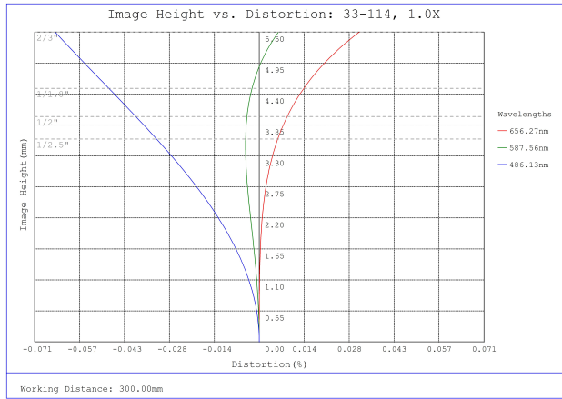
#33-114, 1X, 300mm WD, In-Line CompactTL™ Telecentric Lens, Distortion Plot
