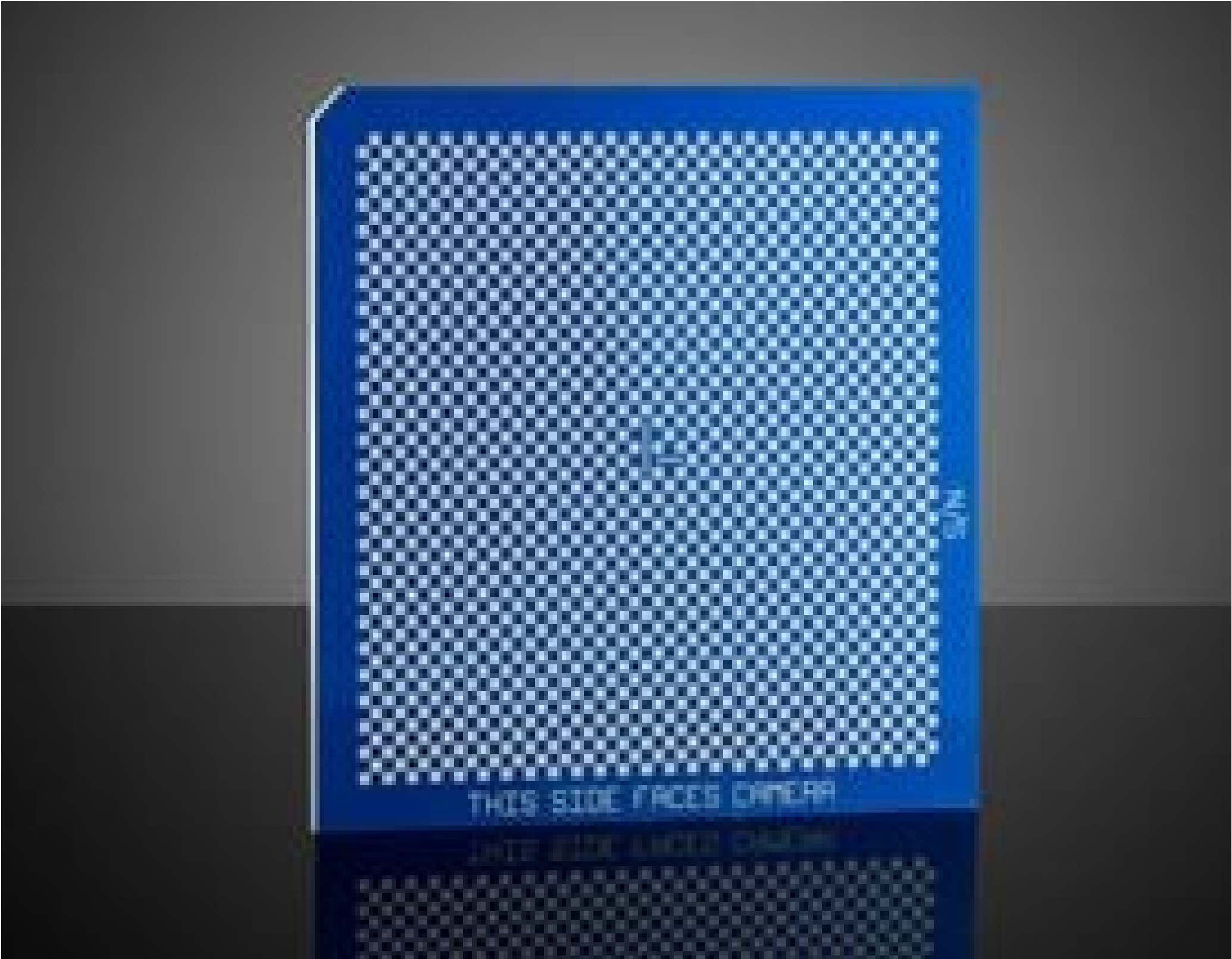
Opal Checkerboard Calibration Target
