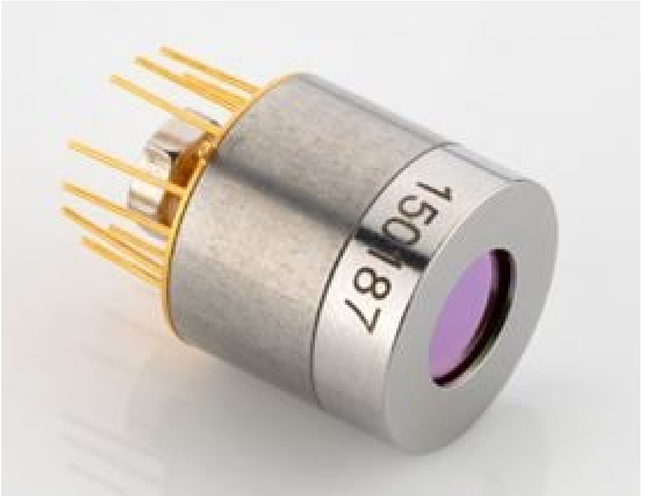
2.2 - 13.6um InAsSb Photovoltaic Infrared Detector, PMA-4TE-13-1x1-TO8-wZnSeAR36
