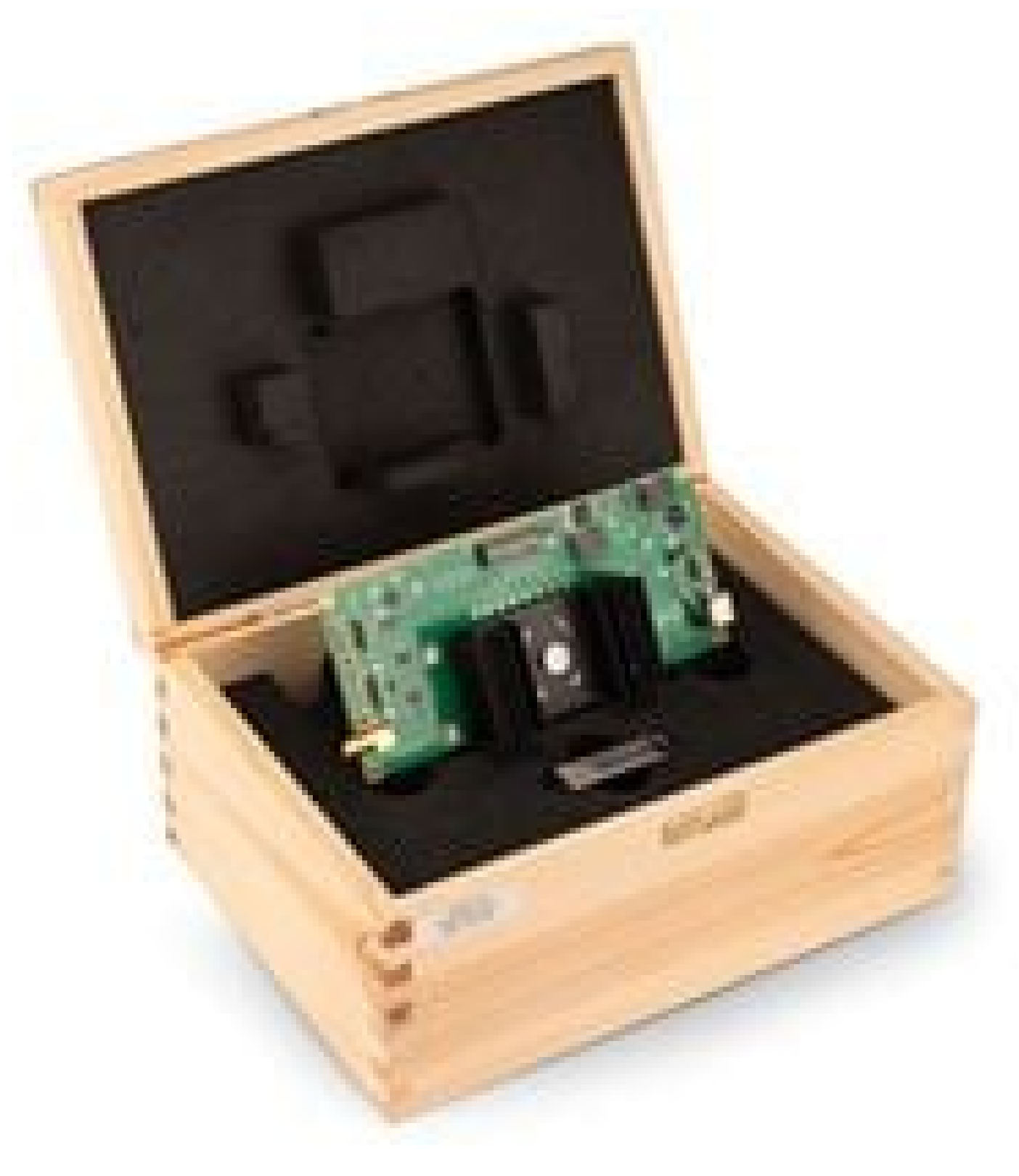
2.2 - 5.5um HgCdTe Photovoltaic Detector Module, AMS3140-01
