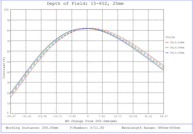
#15-652, 25mm, f/11 Cw Series Fixed Focal Length Lens, Depth of Field Plot, 200mm Working Distance, f11
