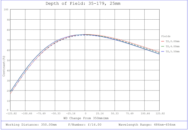
#35-179, 25mm, f/16 Cr Series Fixed Focal Length Lens, Depth of Field Plot, 350mm Working Distance, f16
