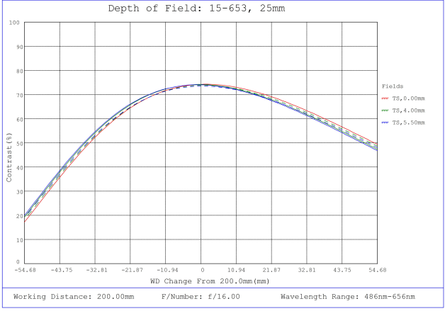
#15-653, 25mm, f/16 Cw Series Fixed Focal Length Lens, Depth of Field Plot, 200mm Working Distance, f16
