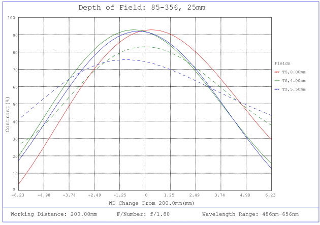
#85-356, 25mm, f/1.8 Ci Series Fixed Focal Length Lens, Depth of Field Plot, 200mm Working Distance, f1.8
