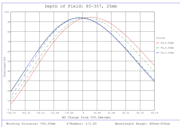
#85-357, 25mm, f/2.8 Ci Series Fixed Focal Length Lens, Depth of Field Plot, 500mm Working Distance, f2.8
