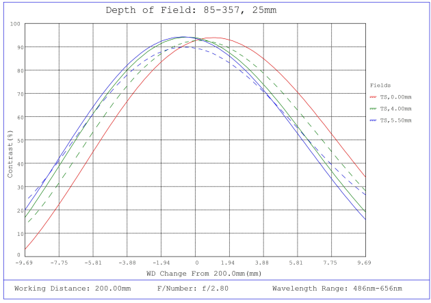
#85-357, 25mm, f/2.8 Ci Series Fixed Focal Length Lens, Depth of Field Plot, 200mm Working Distance, f2.8
