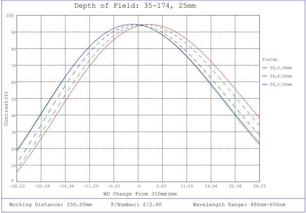
#35-174, 25mm, f/2.8 Cr Series Fixed Focal Length Lens, Depth of Field Plot, 350mm Working Distance, f2.8
