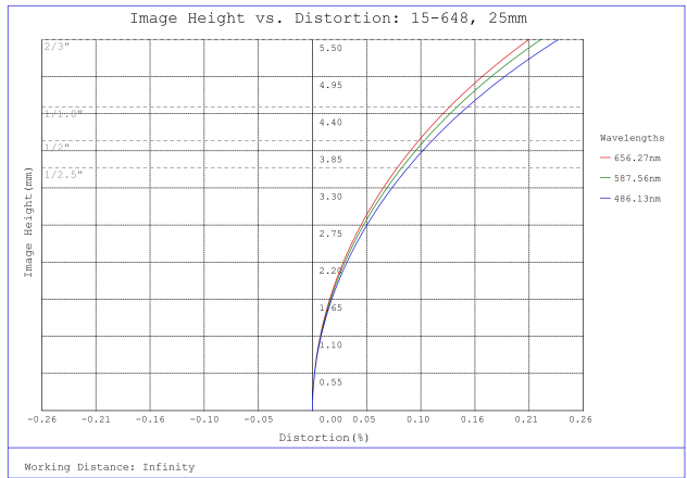
#15-648, 25mm, f/2.8 Cw Series Fixed Focal Length Lens, Distortion Plot
