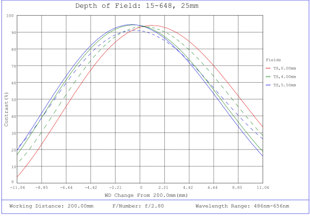
#15-648, 25mm, f/2.8 Cw Series Fixed Focal Length Lens, Depth of Field Plot, 200mm Working Distance, f2.8
